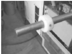
1. Place bar support collar around barstock. Tighten set screw.
